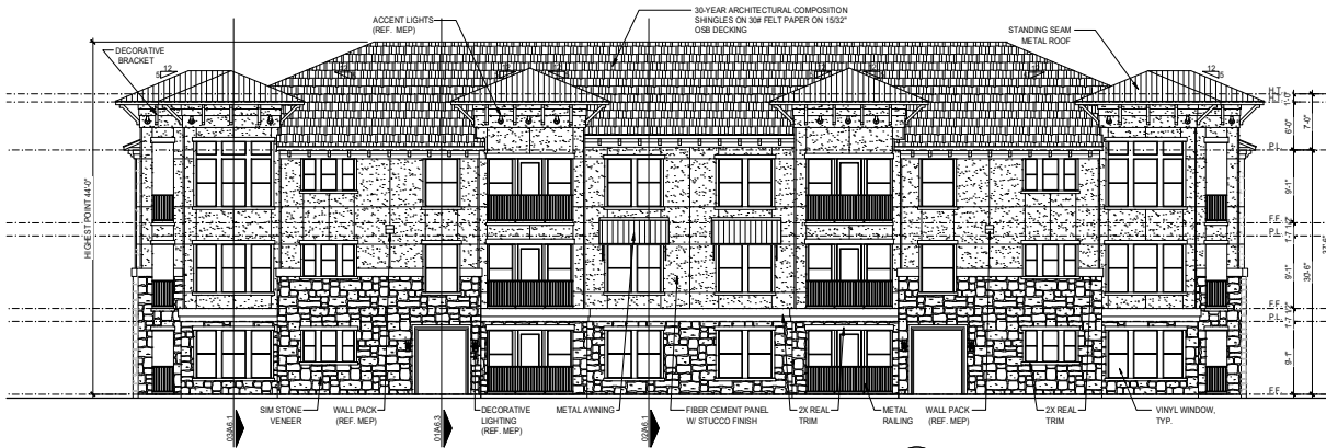
04 BUILDING TYPE 'B' REAR ELEVATION SCALE: 1/8" = 1'-0" 10 REQ'D
