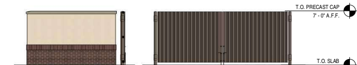
5 OVERALL FRONT & SIDE TRASH ENCLOSURE ELEVATIONS Scale: 1/8" = 1'-0"
