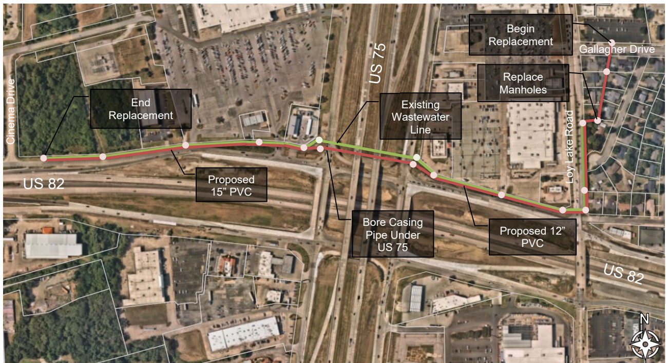
Figure 2: Proposed conditions for wastewater line replacement.
