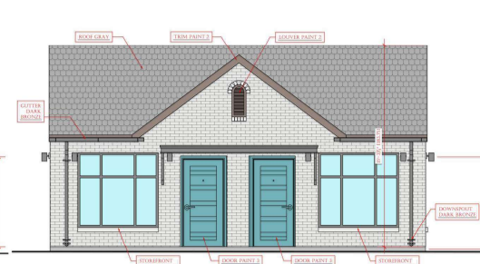
05 NORTH BUILDING EAST ELEVATION SCALE: 1/4"=1'-0"
