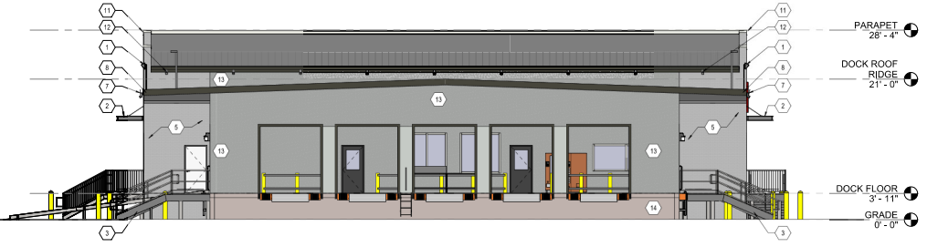
4 TERMINAL SOUTH ELEVATION 1/8" = 1'-0"
