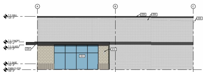
04 EXTERIOR SOUTH ELEVATION (SIDE) SCALE: 1/8" = 1'-0"
