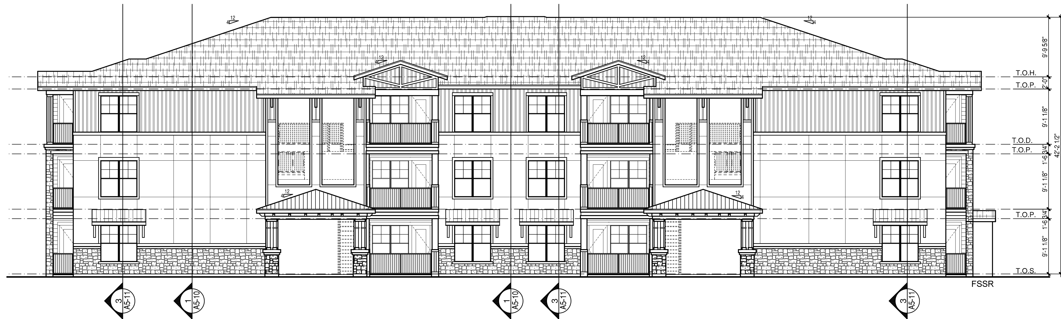
1 BUILDING TYPE 'C' FRONT ELEVATION SCALE: 1/8" = 1'-0"
