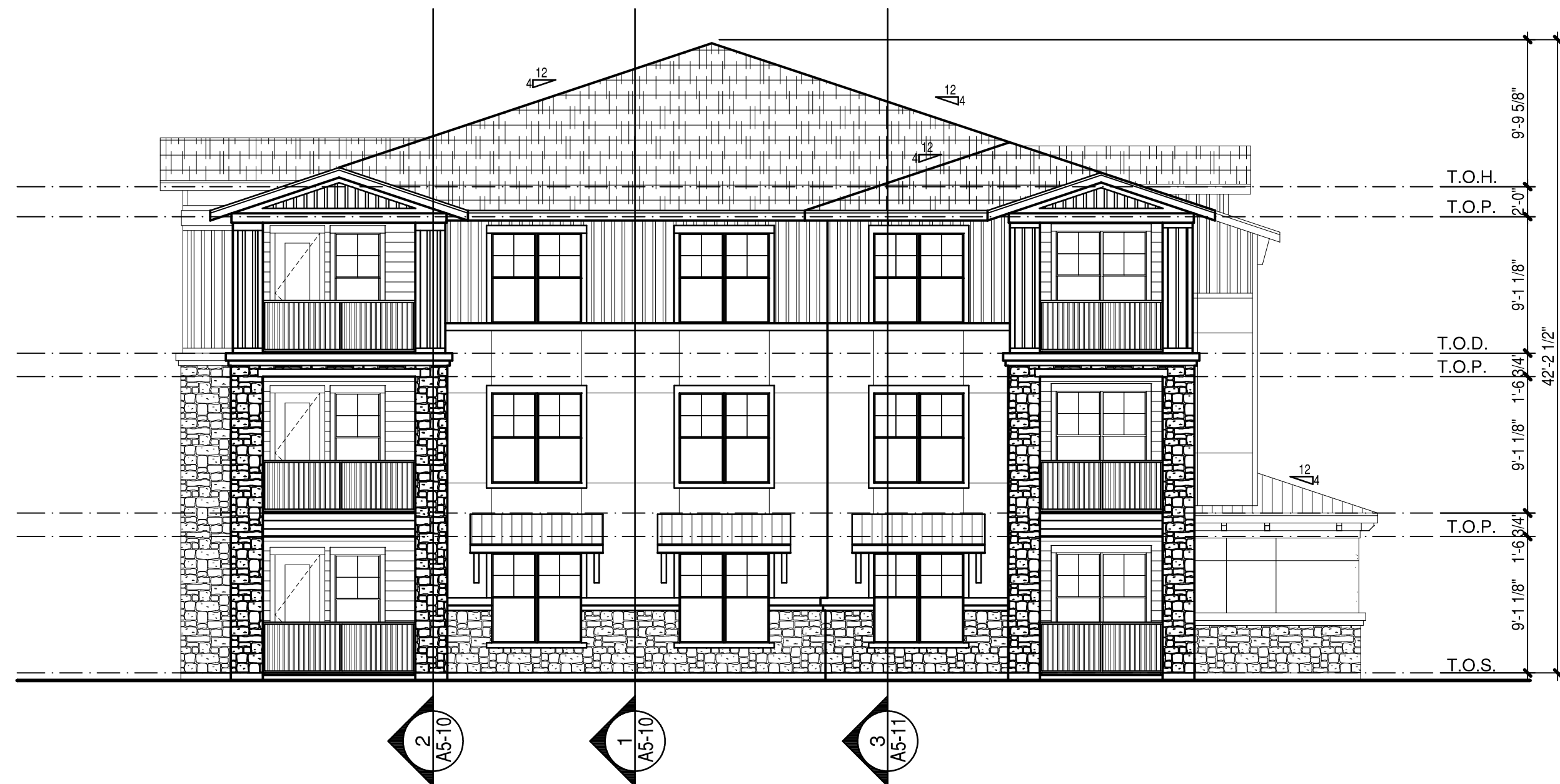
2 BUILDING TYPE 'C' END ELEVATION SCALE: 1/8" = 1'-0"
