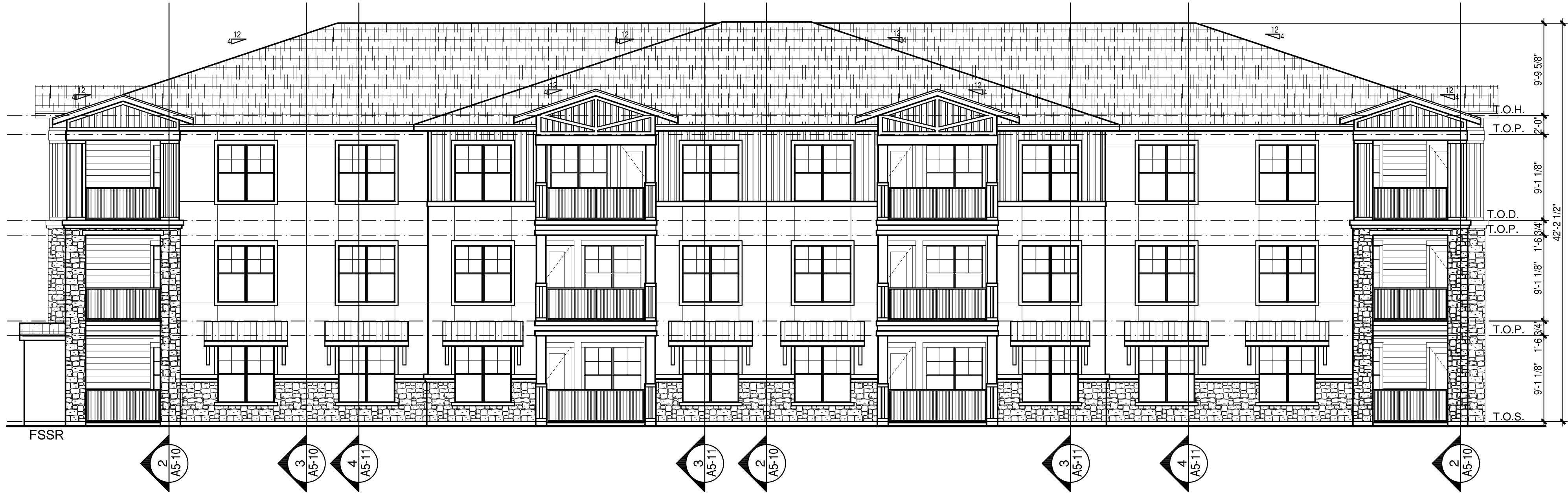
1 BUILDING TYPE 'C' REAR ELEVATION SCALE: 1/8" = 1'-0"
