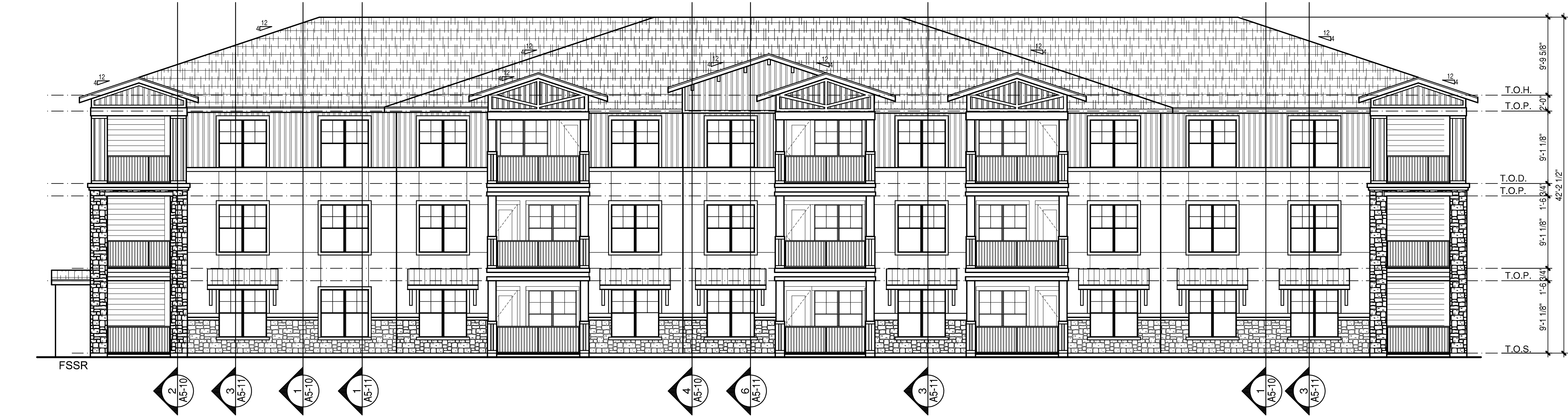
1 BUILDING TYPE 'B' REAR ELEVATION SCALE: 1/8" = 1'-0"
