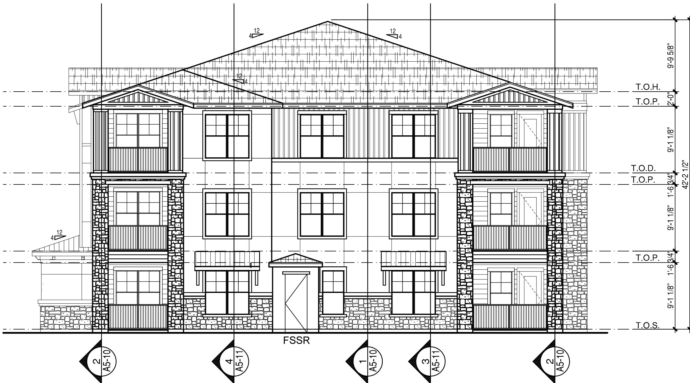
3 BUILDING TYPE 'B' END ELEVATION SCALE: 1/8" = 1'-0"
