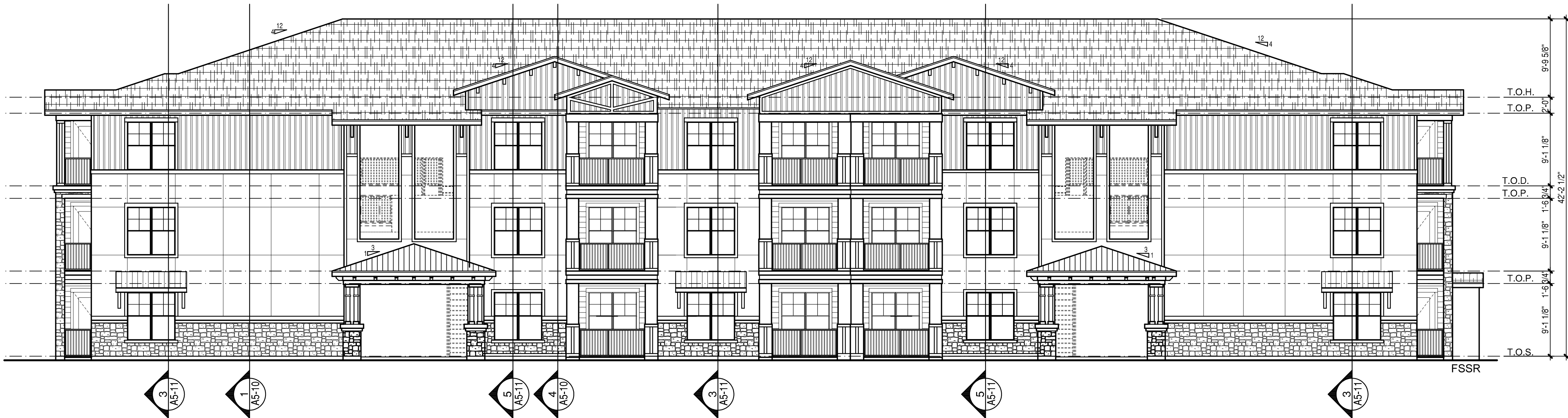
1 BUILDING TYPE 'B' FRONT ELEVATION SCALE: 1/8" = 1'-0"
